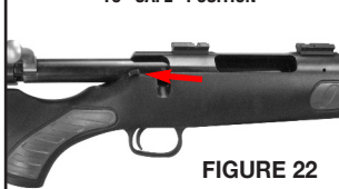
PUSH SAFETY LEVER FULLY REARWARD TO “SAFE” POSITION
