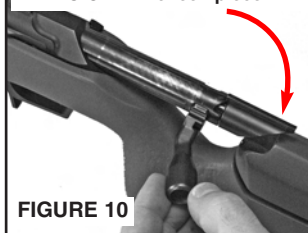
ROTATE BOLT UPSIDE DOWN TO CLEAR cheek piece
