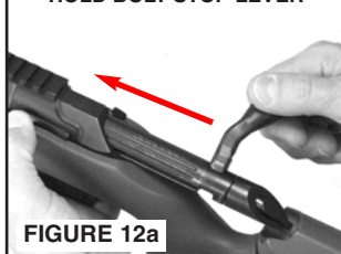
PUSH THE BOLT IN - AS YOU HOLD BOLT STOP LEVER
